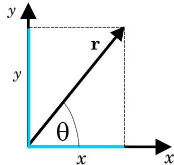
**Figure 4.3** The rectangular components of a vector.
